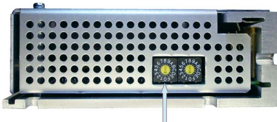
Set the address in hex values. For any address up to 15, keep the left rotary switch on zero. For higher addresses, multiply the left rotary switch setting by 16 and add to the value on the right.
