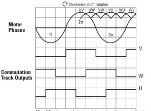
Max. Misalignment between rising edge of commutation track V & zero crossing of back EMF UV  $<=5^{\circ}$  electrical.
