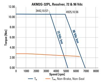
$$\begin{split} T_p &= \text{Peak torque} \\ T_{mc} &= \text{Maximum continuous torque} \end{split}$$
